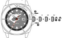
After setting of current date, time and winding of the watch put the winding crown back in the neutral position by pressing it in a direction to the case and put it back in the safe/screwed position by rotating it in a clockwise direction. Only in such a position of the winding crown water resistance at depth down to 200 m is guaranteed
