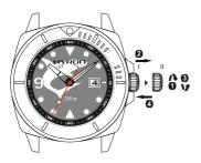
WARNING: IF YOU CONTINUE WINDING THE WATCH AFTER YOU FELT THE RESISTANCE, THERE IS A RISK OF BREAKING THE TIP OF THE SPRING. IN THIS CASE, REPLACEMENT OF THE BARREL DRUM AT THE EXPENCE OF THE OWNER WILL BE REOUIRED.
